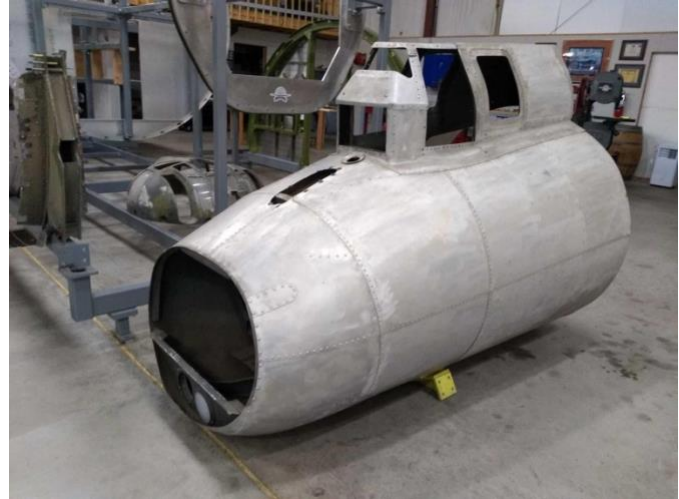
The “new” Lucky Thirteen stinger, after clean-up
