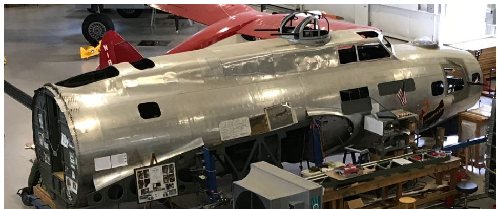
A close-up view of Champaign Lady's forward fuselage assembly, under construction.
