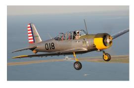
In August 1942, I was reassigned to Bakersfield, CA and flew the Vultee BT13 – 450 hp with radio and adjustable prop. Quite a hot rod after the Ryan.
