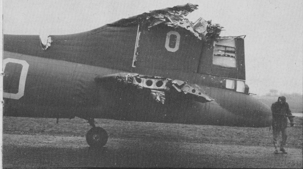
Raedeke's B-17, most of its tail smashed away, back home after the loop.
