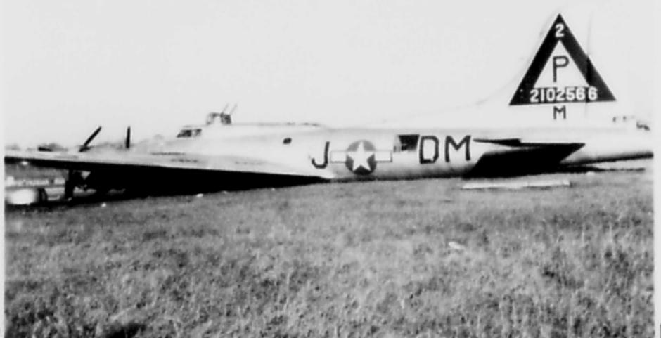
(GAD-88-2-384) (21-Nov-44) 2102566. Landing Gear Failure
